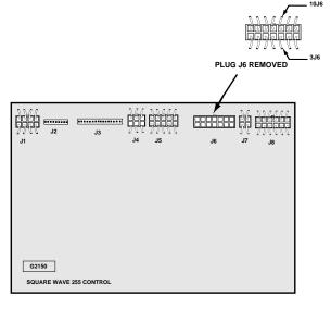
FIGURE F.8 - CONTROL BOARD TEST POINTS.
